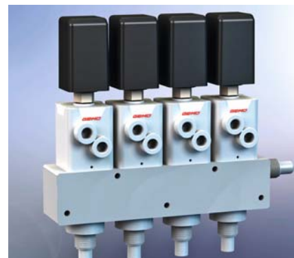
4-way block in PTFE with flare connections, pneumatic actuators type GEMÜ C50 and GEMÜ 1234 electrical position indicators
