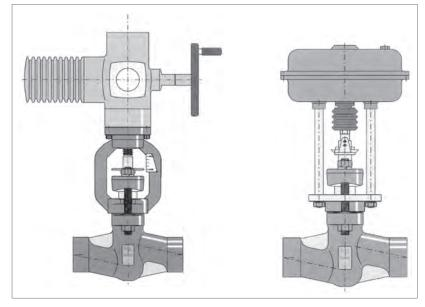
This valve type can be supplied with electrical or mechanical position indication, pneumatic or electric actuator, a locking device for open-closed position. See below.
